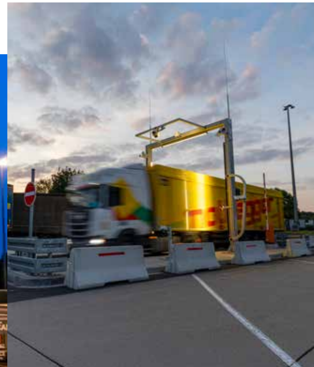
Every day, about 900 trucks and their containers are registered seamlessly by Camco’s entrance gates in Cologne – the result of hardware and software working hand in hand.
