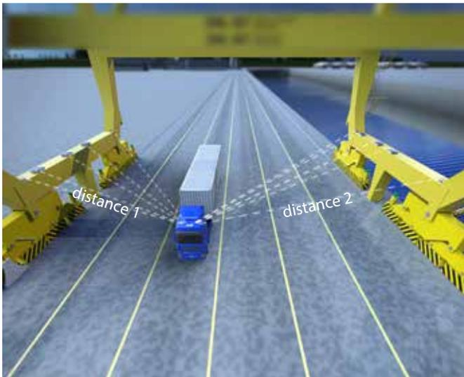
Here, micro location technology can fill the gap. This technology is based on distance ranging by the use of low power 500 Mhz wide pulses in the unlicensed 3 to 8 Ghz band, called UWB-IR. Due to its centimeter accuracy and low energy it is used in high-end drones.
