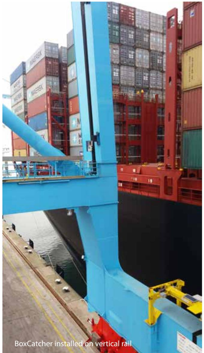
BoxCatcher installed on vertical rail
